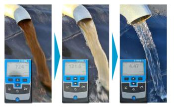
Checks of the turbidity values provide clear information about the progress and success of the cleaning process.
