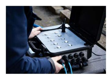
In the MTA Roof Scan® software, you can see the values measured between 2 probes in real time - this makes it very easy to locate leaks.
