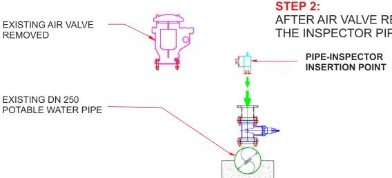
AFTER AIR VALVE REMOVAL INSERT THE INSPECTOR PIPE MACHINE
