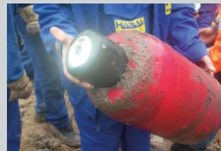
MTA Pipe-Inspector® in pipe pig
