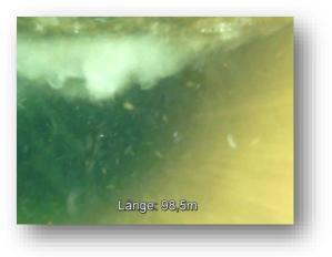
Air pockets can lead to problems during the inspection for which the Contractor cannot be held liable. This does not constitute an impairment of the results of the inspection.
