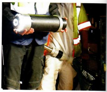
MTA Pipe-Inspector DN125 continues to operate after extraction until turned off and on-board data extracted to computer for immediate video review and data analysis
